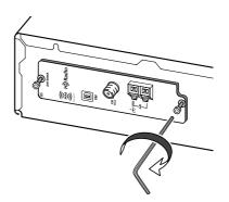
Be sure to fully tighten the screws. If they are loose, the ground connection between the board and the T-4555P may be inadequate, resulting in noise or failure.
